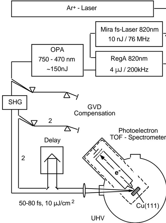
Figure 2: Experimental setup for time-resolved photoemission. An optical parametric amplifier (OPA) outputs tunable femtosecond laser pulses, which are delayed with respect to the second harmonic (SHG) pulses ( $2\omega$ ) are delayed with respect to the fundamental ( $\omega$ ) pulses and focused onto the Cu(111) sample. The photoelectrons are detected in a time-of-flight (TOF) spectrometer.
