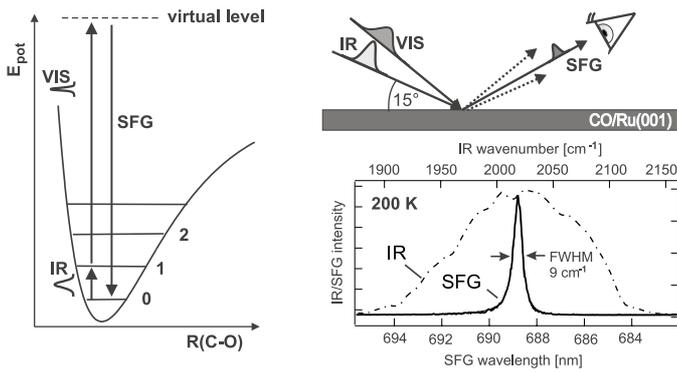
**Fig. 7** Left: Principle of IR-VIS-SFG (see text). Right top: Scheme for broadband-SFG. Right bottom: SFG spectrum of the CO stretch vibration of  $(\sqrt{3}\times\sqrt{3})$ -CO/Ru(001) at 200 K (black line). The spectrum of the broadband-IR pulse is shown as dashed curve. **FIGURE 7: TWO COLUMNS**
