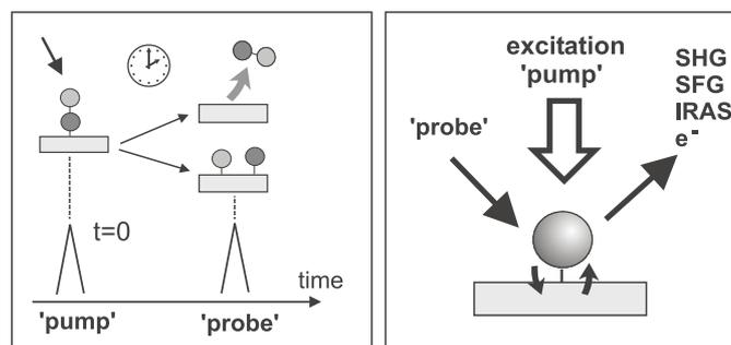
**Fig. 6** Methods of time-resolved spectroscopy on surfaces based on the pump-probe technique: An ultrafast laser pulse ('pump') initiates a reaction of adsorbed molecules. Changes in the adsorbate-substrate system are monitored at later times with a second ultrafast laser pulse ('probe').
