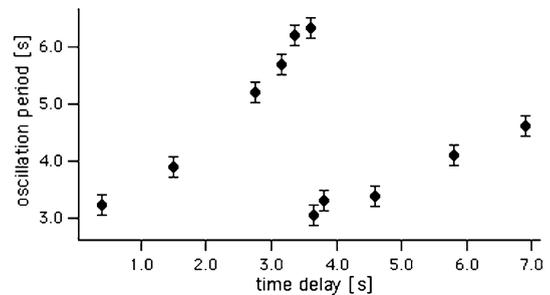
Fig. 2. Oscillation period of the forced system for different time delays. The rapid decrease of the period at  $\tau = 3.7$  s marks the transition from desynchronization to synchronization ( $\mu = 0.4 \times 10^{-5}$  mbar).
